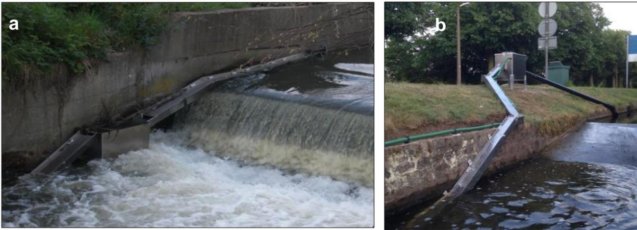
Figure 5: Two of the different types of traps used for monitoring. (a) a gravity supplied trap at Hogsmill-Middle Mill, and (b) a pumped trap at Crane-Mogden Sewage Treatment Works (STW).
